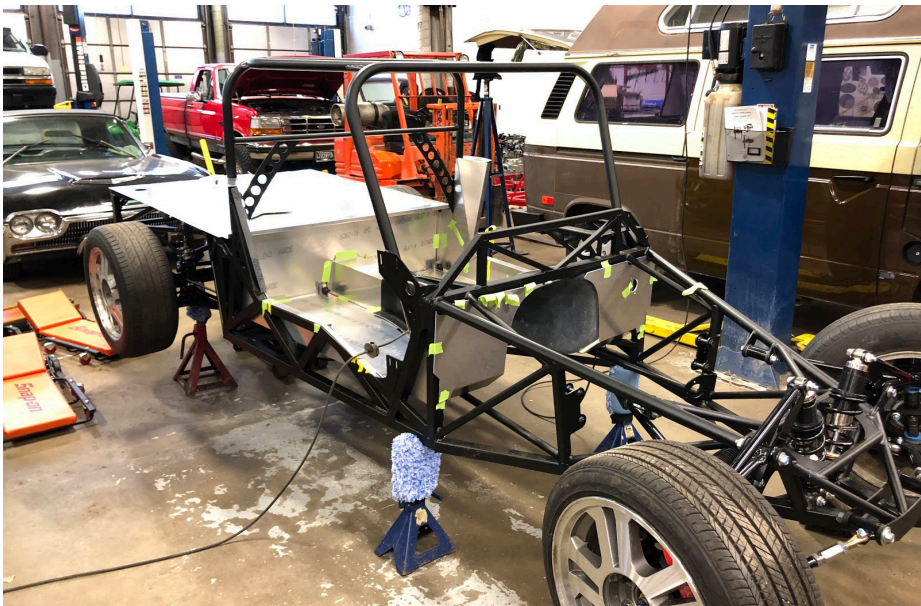
1935 Factory Five Kit car in the process of being built. Photo by Sache Krishnaraj
